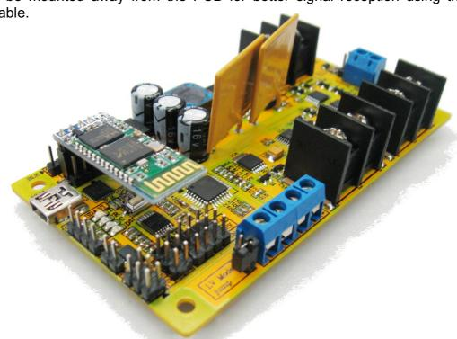
If the bluetooth module is detected the sample code will automatically set the baud rate to 9600, the name to "T'REX" and the pin number to "1234".
