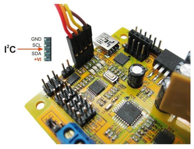
Connect the +V, SCL, SDA and Gnd of the external logic to the +VI, SCL, SDA and GND pins of the T'REX I²C interface. The T'REX will automatically translate the voltage. The interface includes 10K pullup resistors although external pullup resistors can be added if required.
