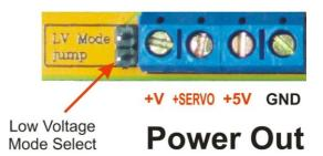
The 5V regulator will get much hotter in this mode so the 5V current should be limited to 800mA unless a heatsink and fan are added directly to the LM1084 regulator IC.
